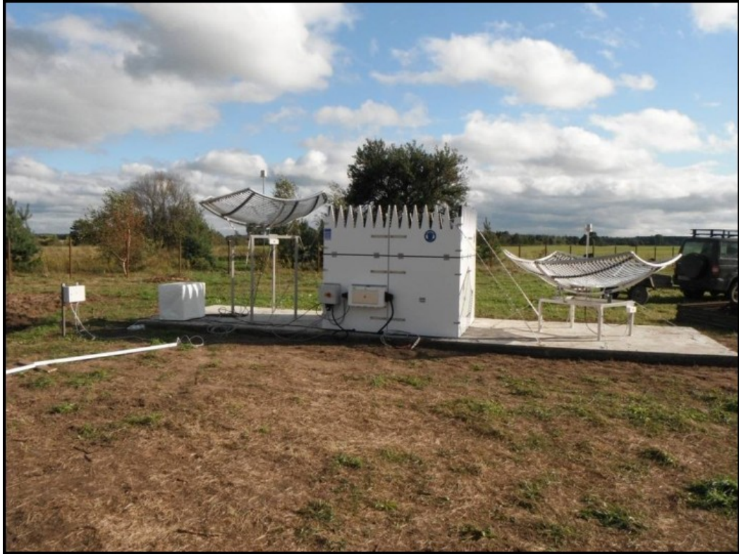
Figure 8.17 – SODAR measuring complex
