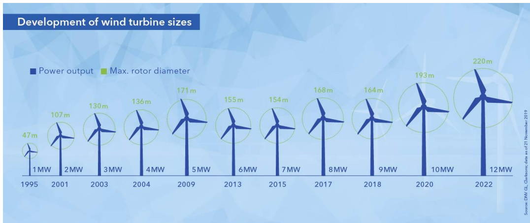
Figure 3. The development of wind turbine size and capacity between the years 1995 and 2022 (DNV). In 2023, the installed wind turbine capacity was 15 MW.
