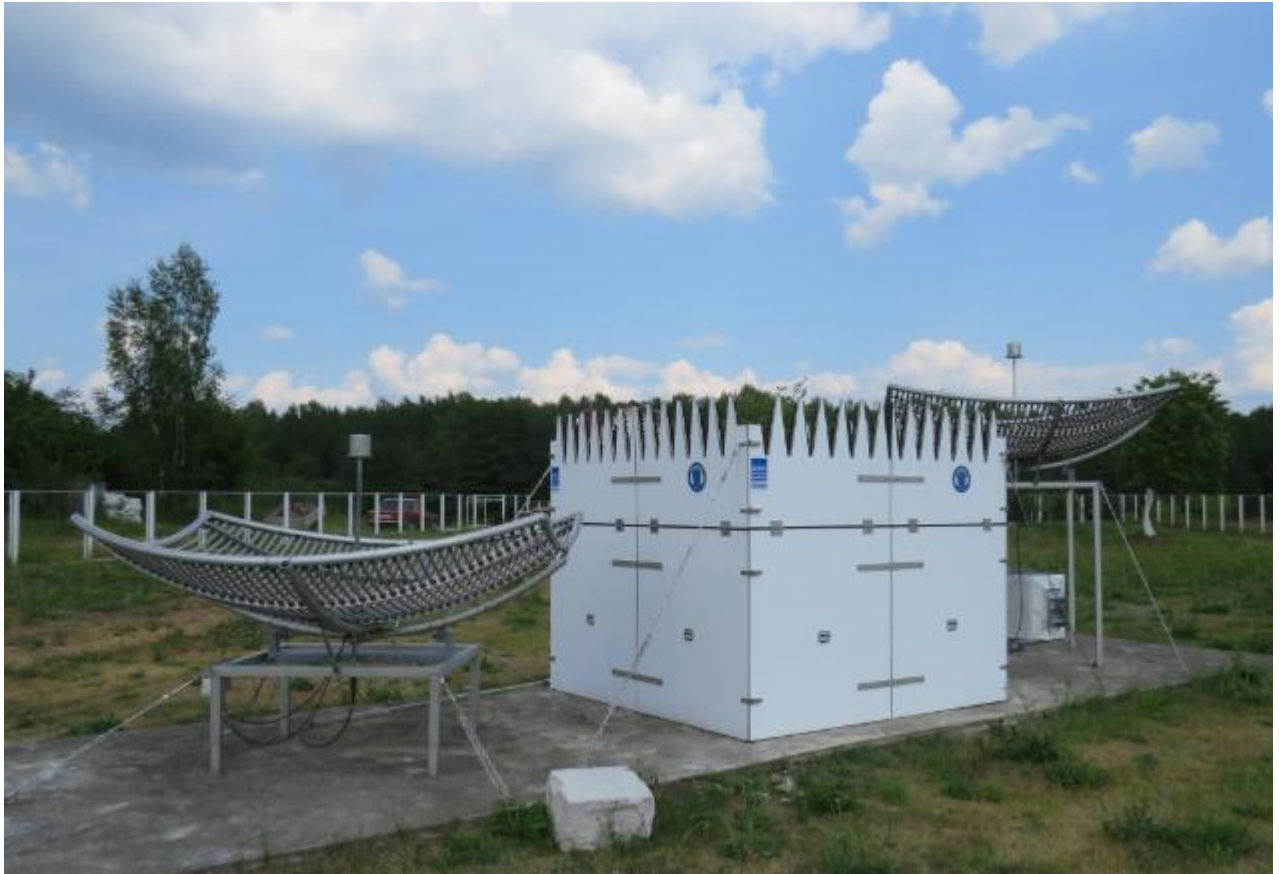
Figure 8.17- SODAR measuring complex
