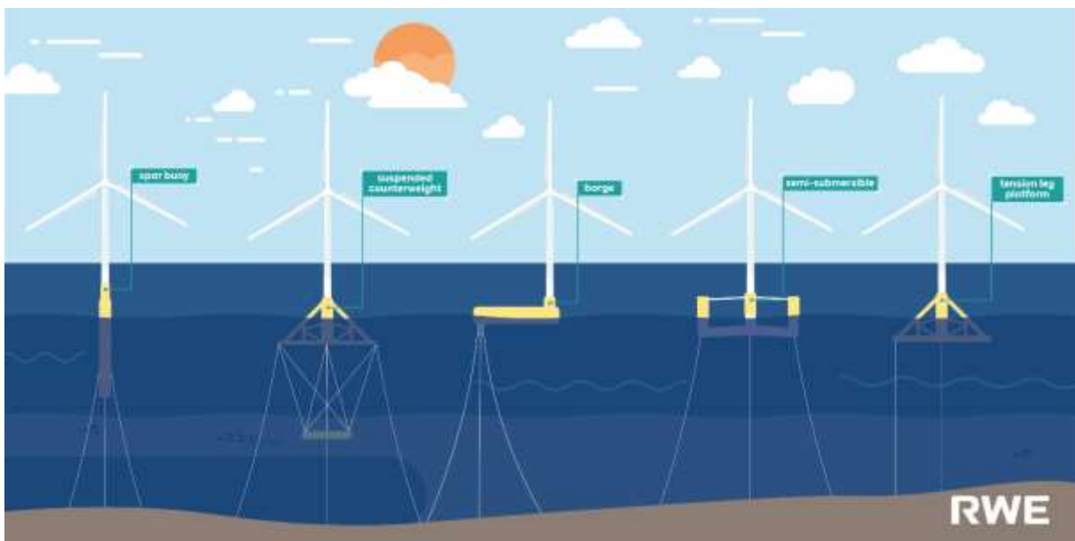
Figure 5. Different types of floating foundations.
