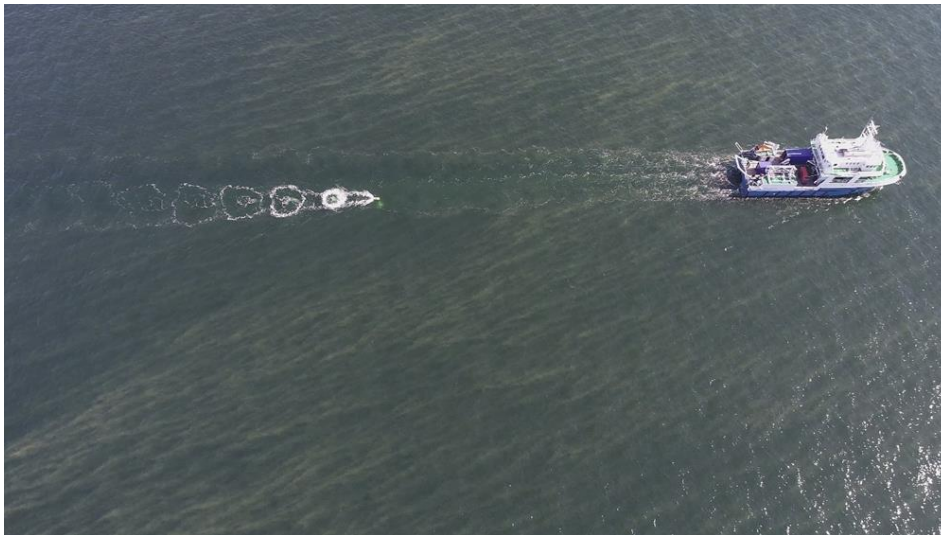
Figure 4-1 The picture shows SGU's vessel S/V Ocean Surveyor during seismic measurements south of Scania in 2023. The picture uses an air cannon that is visible just over two boat lengths behind the vessel.
