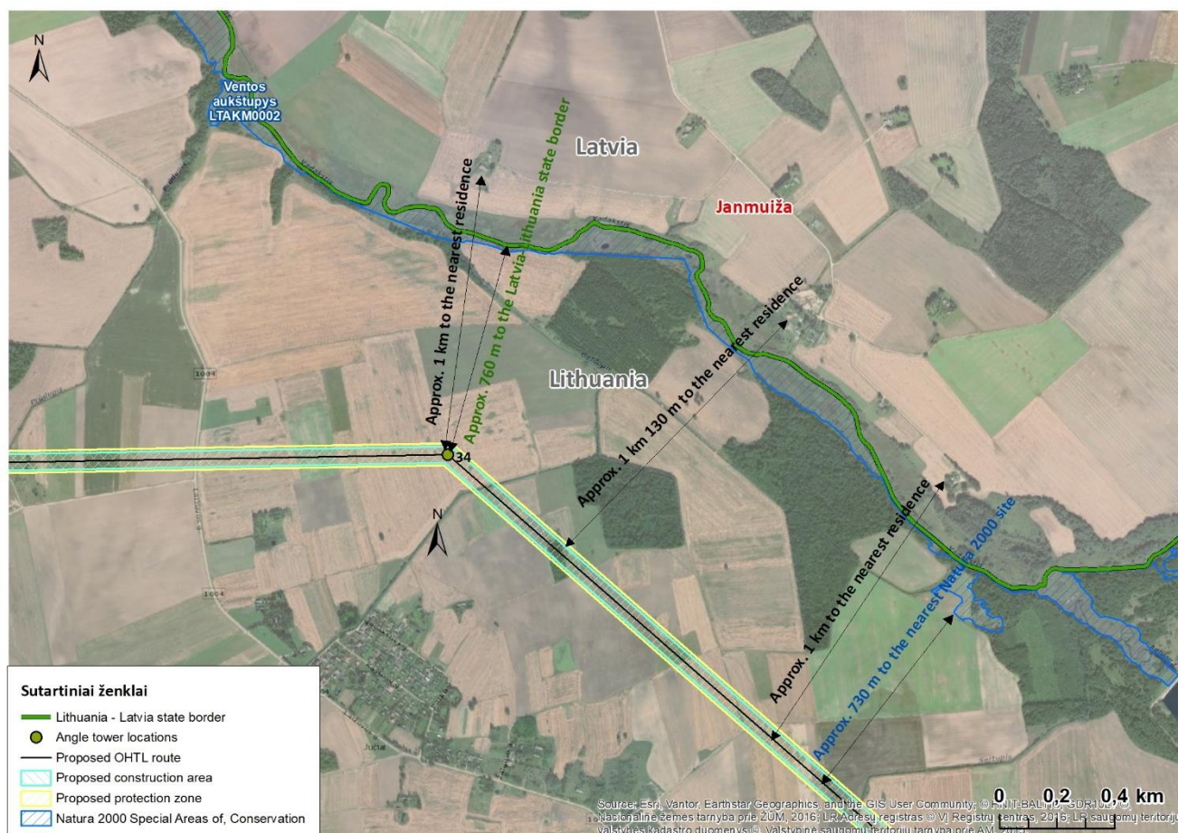
3 pav. Section of the Proposed Overhead Transmission Line Route Closest to the State Border between the Republic of Lithuania and the Republic of Latvia, Including the Distances to the Nearest Residential Buildings and Natura 2000 Sites
