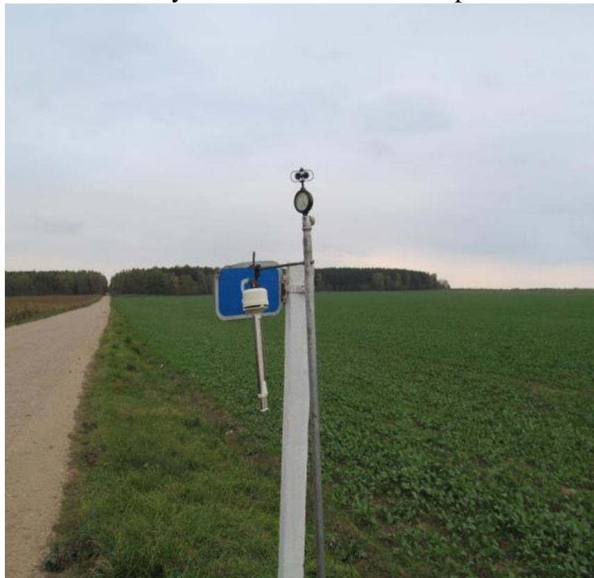
Figure 8.11 - Microclimate monitoring point
